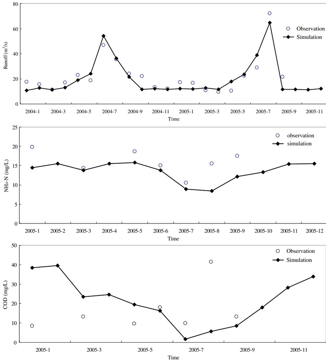
**Fig. 5** Monthly observed and simulated runoff and  $\text{NH}_4\text{-N}$  and  $\text{COD}_{\text{Mn}}$  concentration at Beiguan Floodgate
