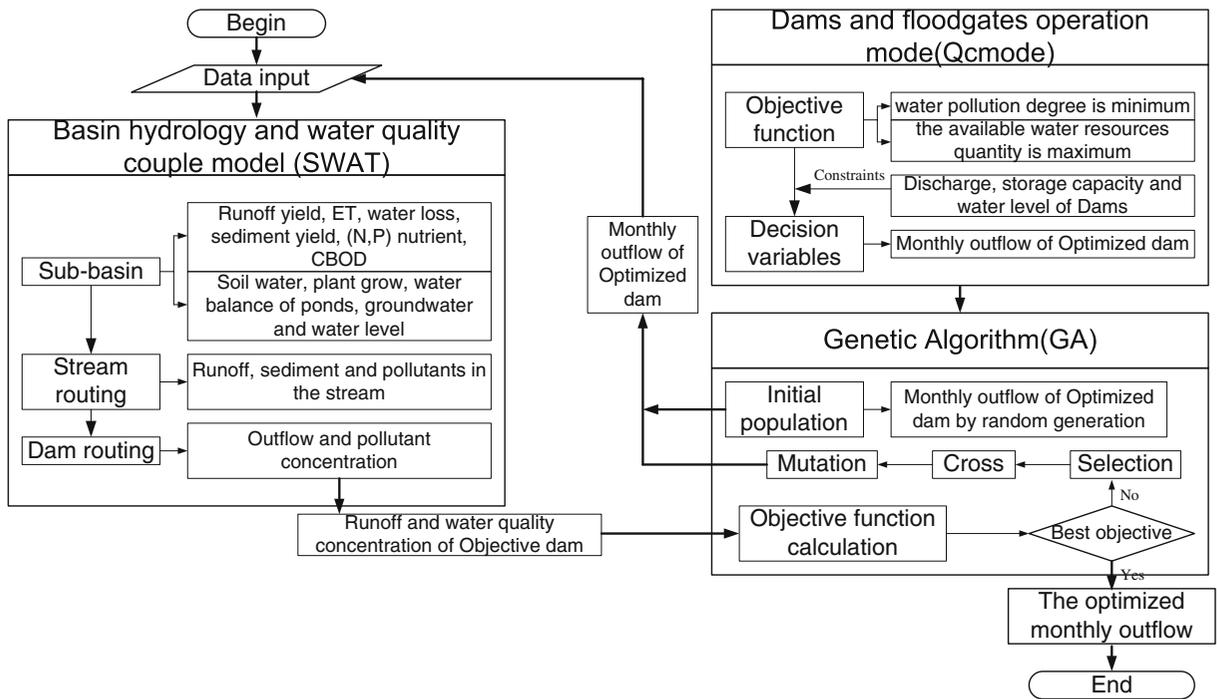
**Fig. 1** SWAT-QCmode model flow chart
