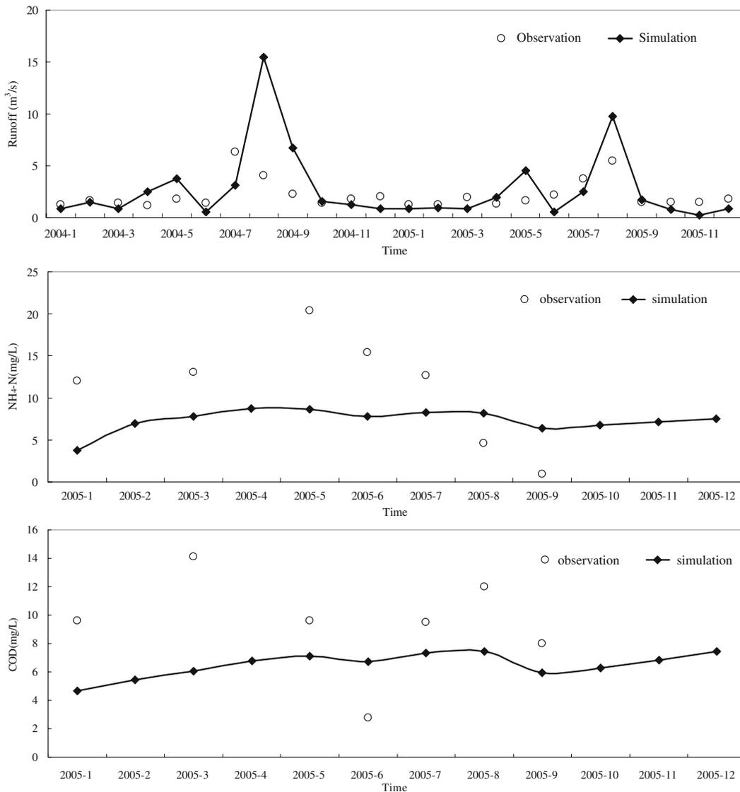
**Fig. 4** Monthly observed and simulated runoff and  $\text{NH}_4\text{-N}$  and  $\text{COD}_{\text{Mn}}$  concentration at Sha River Reservoir
